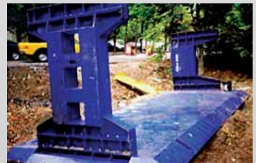
HEAVY DUTY BOLTED SPREADERS FEATURE "WINDOWS" FOR BETTER OPERATOR VIEWING. ADDITIONAL SPACERS CAN BE ADDED FOR WIDTH CHANGES
