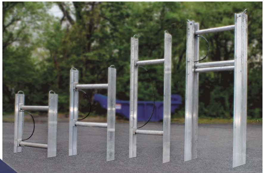
High Clearance Shore - far right- Showing differences from standard shoring
